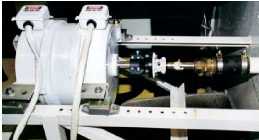
Continuous duty brushless DC permanent magnet (Nd Fe B) the ST 74 is a twin motor that develops 12 nominal horsepowers @1100 rpm (9 kw). Input is 120/144 vdc, with full load amperage at 80/90. Torque 74 lb/ft. Weight 133 lb. Size 13”x17”. Housing is totally enclosed, non-ventilated.
