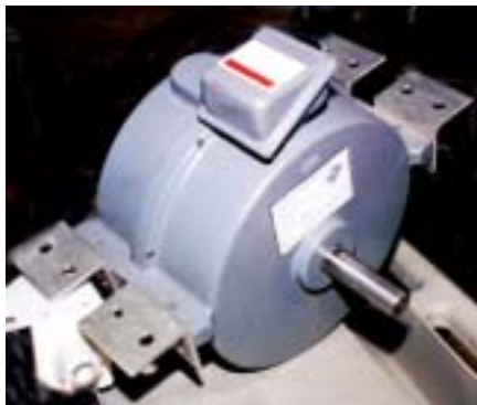
Continuous duty brushless DC permanent magnet (Nd Fe B) the ST 37 is a single motor that develops six nominal horsepowers @1200 rpm (4.5 kw). Input is 144 vdc, with full load amperage is at 32. Torque 37 lb/ft. Weight 98 lb. Size 13”x13”. Housing is totally enclosed, non-ventilated.
